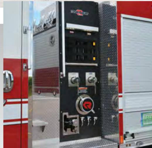
TP3™ Pump Control Panel with Sealed Bank
