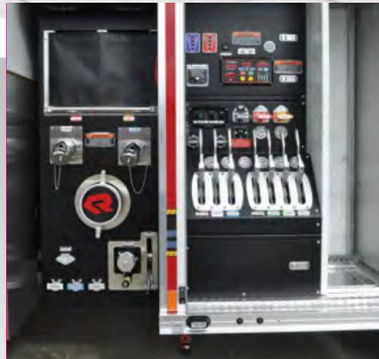
MP3™ Pump Control Panel with Sealed Bank
